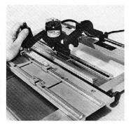
6. With the Motor Mounted Depth Control removed, place the Stylus Tip in the center groove of a 'B, E, F, G, H, P or R' Master Type Letter, or in the center vertically of a 'D, I, K, L, M, N or T.' (Measure and mark the center if necessary.) Loosen the Engraving Position Clamping Knob and slide the Sign Blank Plate until the Cutter point lines up with your pencil center line on the Sign Blank. Tighten the Clamping Knob and replace the Depth Control.
