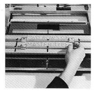
11. The lower row of type is centered either by eye or by using a scale to position it equadistant from the Letterlocks holding the upper row of type. (see photograph)
