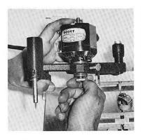
12. Scott Signgravers are shipped from the factory with 1/16" Cutter installed, ready to engrave. To change cutter, first remove the Motor Mounted Depth Control. Place a hex wrench through the hole in the top of the motor shaft to prevent rotation and loosen the Collet Nut. Remove cutter and replace with one of your choice.
