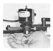
14. Replace the Motor Mounted Depth Control on the Threaded Motor Housing until it locks against the Motor Link of the Pantograph. The Depth Control rides on the surface of the Sign Blank. The amount of cutter that is exposed is the depth of cut. Engrave just deep enough to cut away the surface color. A cut that is too deep can ruin the sign material. It is best to start with a shallow cut, then increase to required depth.
